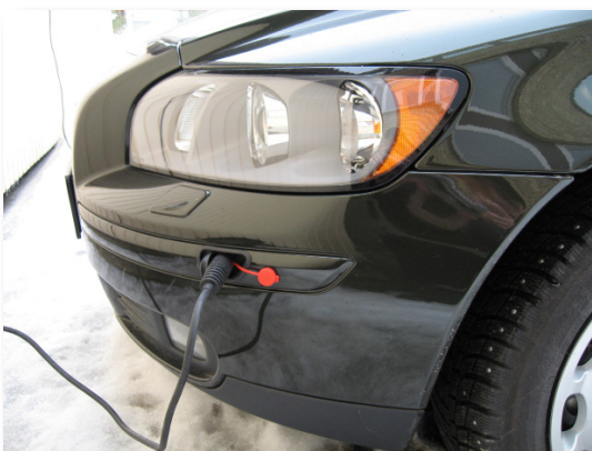
Connecting cable connected to the installed Calix system
