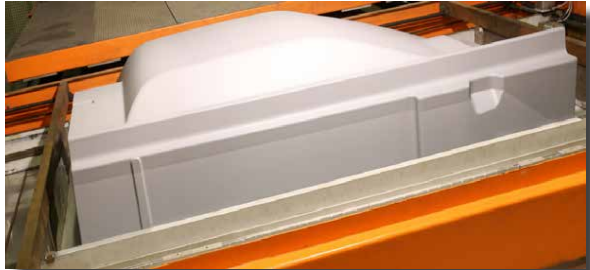
Vacuum-formed interior component
