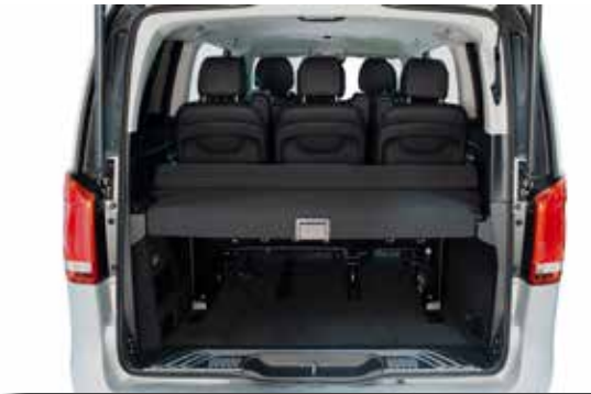
Luggage room divider/bed extender installed in car
