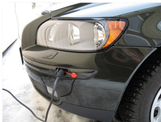
Connecting cable connected to the installed Calix system
