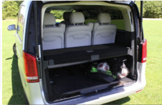
Luggage room divider installed
